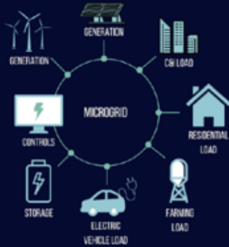
A MICROGRID IS A PHYSICAL ENERGY SYSTEM THAT GENERATES + DISTRIBUTES ELECTRICITY WITHIN ITS OWN GEOGRAPHIC FOOTPRINT.
